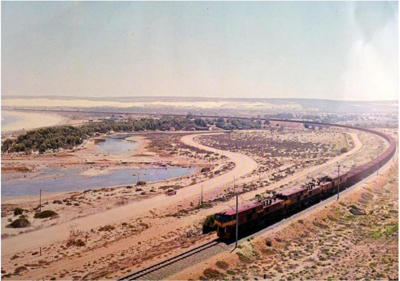
Fig. 3. Long-haul iron ore train on Sishen–Saldanha Orex line in South Africa, pulled by electric locomotives under 50 kV catenary. (Photo: Peter Ball collection, http://www.theheritageportal.co.za/article/south-africas-world-record-breaking-train )
