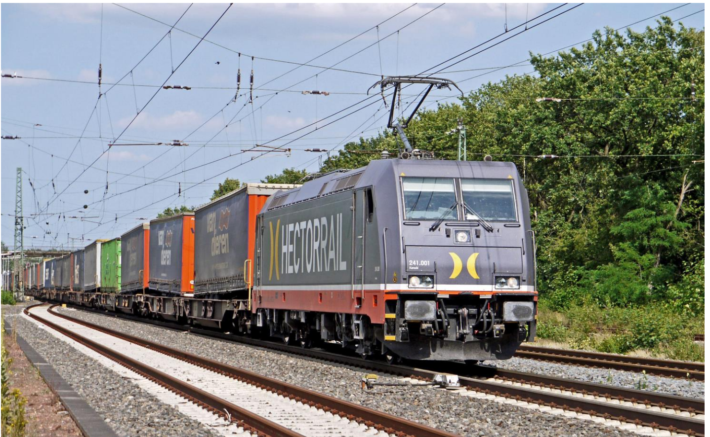
Hector Rail intermodal freight train in Germany, pulled by Bombardier TRAXX electric locomotive (Photo: pxhere.com, Creative Commons CC0)
