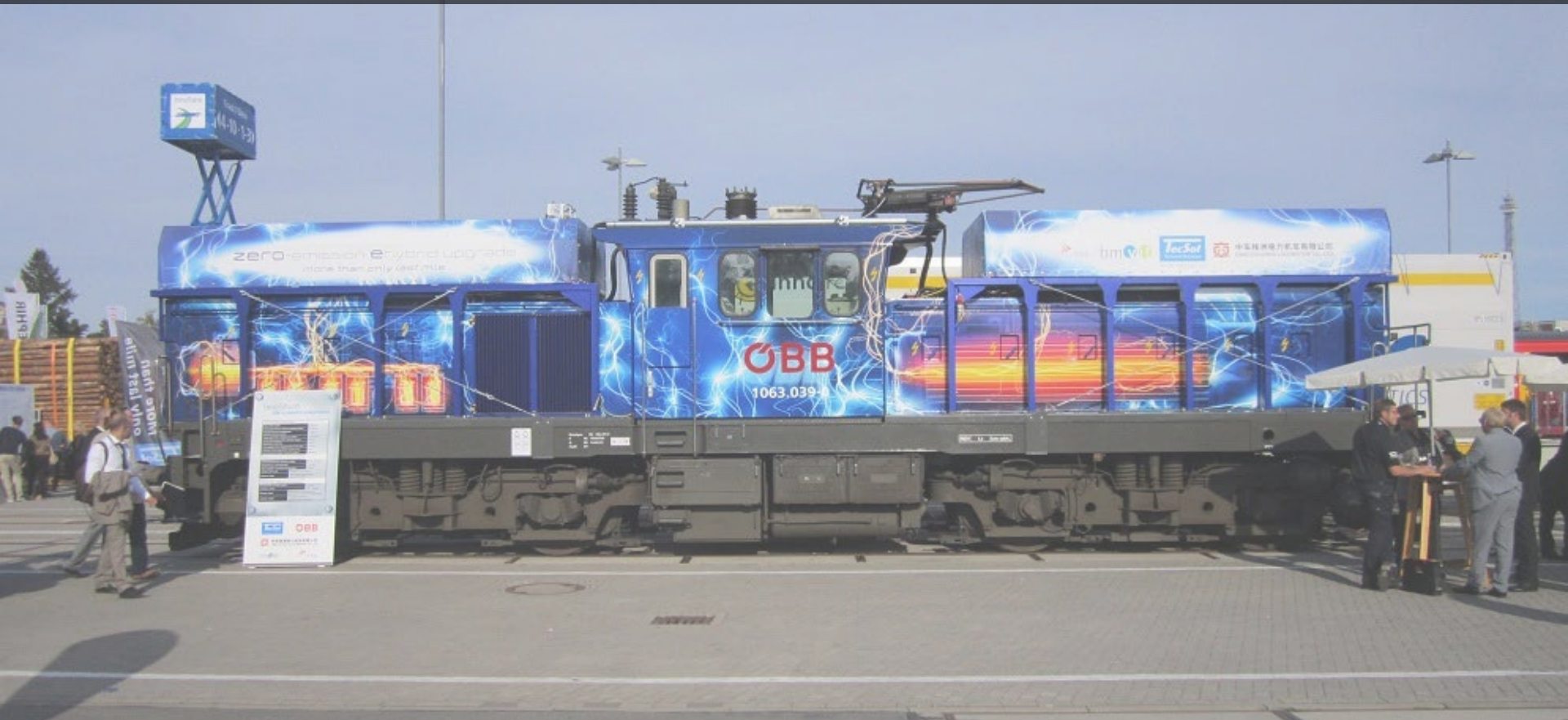
Austrian Federal Railways ÖBB InnoShunt eHybrid prototype catenary-supercapacitor-battery switcher. Rebuild of Class 1063 electric locomotive by vehicle modernisation company TecSol
