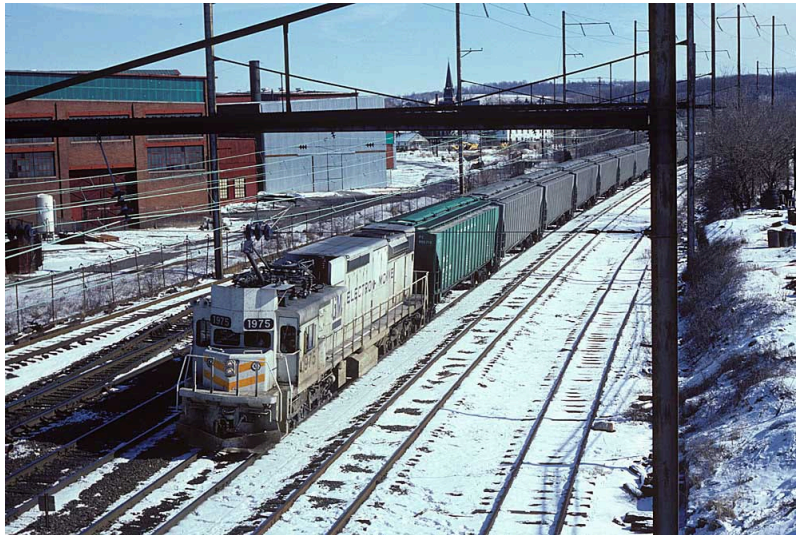
“When they did get to run, the EMD freight electric locomotives showed the designs were more than viable”: 6,000 hp GM6C on Conrail, Feb. 11, 1979, at Middletown, Pennsylvania (photo: Stephen J. Salamon , David P. Oroszi collection), from “Testing EMD electric freight locomotives”, by Preston Cook, May 31, 2022, Trains.com: https://www.trains.com/ctr/railroads/locomotives/testing-emd-electric-freight-locomotives/
