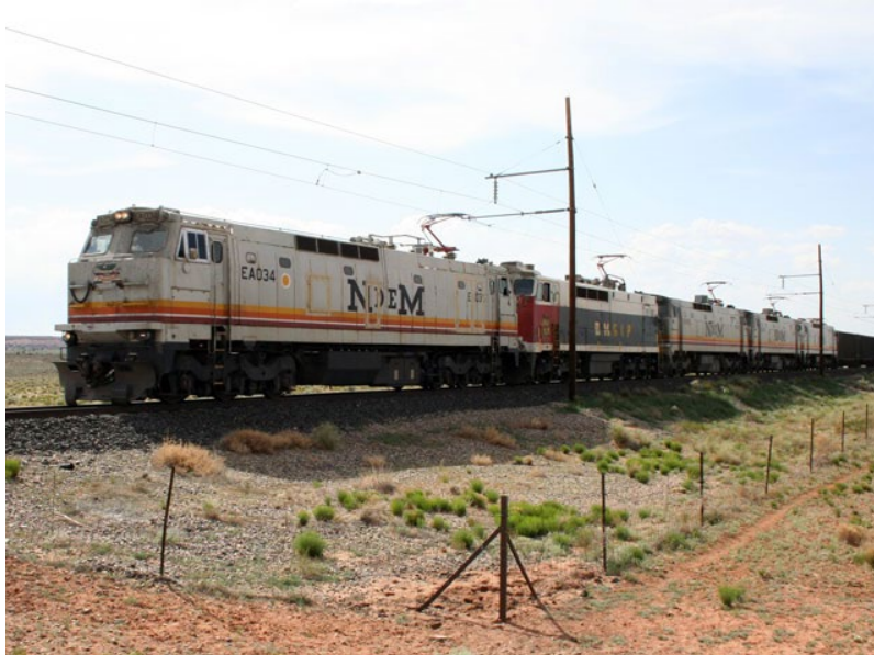
Arizona’s Black Mesa & Lake Powell Railroad electric General Electric (Wabtec) E60 50 kV 6,000 hp locomotives, which ran from 1973 to 2019
