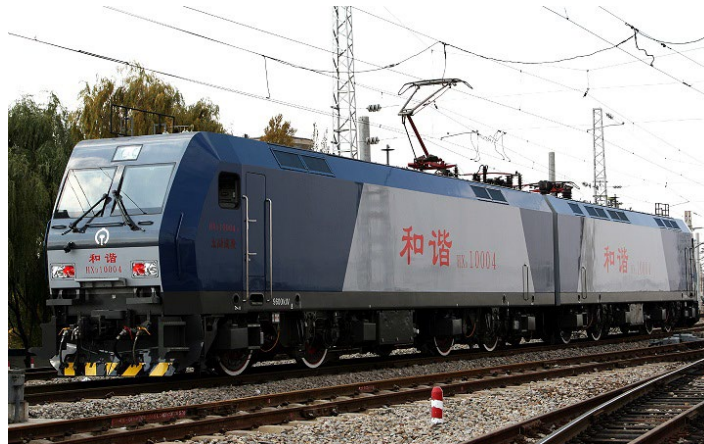
One of the world's most powerful locomotives: China Railway HXD1 series 12,900 hp freight two unit locomotive set, which by itself under 25 kV overhead catenary wire pulls 20,000 ton trains (Photo: https://commons.wikimedia.org/wiki/File:HXD10004.jpg )
