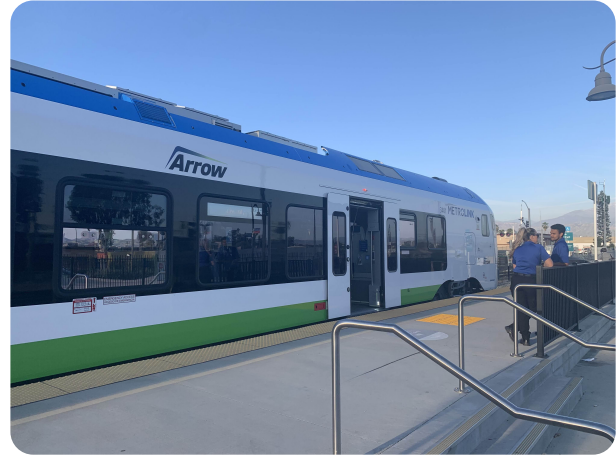
Level boarding at an Arrow train at the San Bernardino Station Metrolink station. Notice the platform height is level with the train floor.
